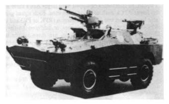
Figure 6-4. BRDM reconnaissance cars. These wheeled armored vehicles appear in numerous variations, including ATGM launchers and CBR reconnaissance cars. They are found in almost all Soviet reconnaissance units. The older BRDM (above) is probably being phased out in favor of the BRDM-2 (below) which mounts a turret similar to the BTR-60 PB.
